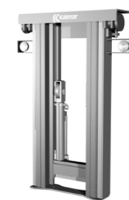
Triplex full free lift, free visibility
