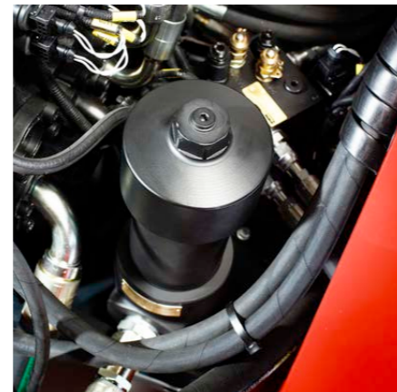
Improved placement of hydraulic filters.
