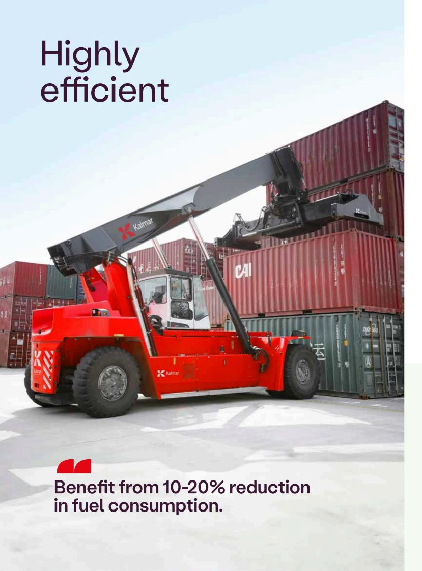
Our Essential Reachstacker comes fitted with load sensing hydraulics and there is a range of the latest generation of engines and transmissions to choose from. You will get a highly efficient and powerful machine that uses less fuel, produces less emissions, costing you less, while maintaining productivity.
