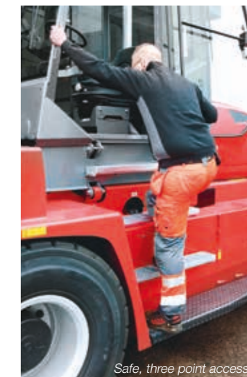
Safe, three point access.
