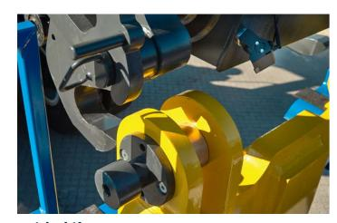
**Quick shift** Custom-made quick-shift solution, where only 2 persons can easily shift between hook and spreader. The work platform has a built-in hook-mount.
