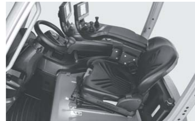
Swivel seat for comfortable reversing
