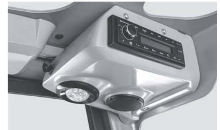
Reading light and radio with hands-free system and speakers
