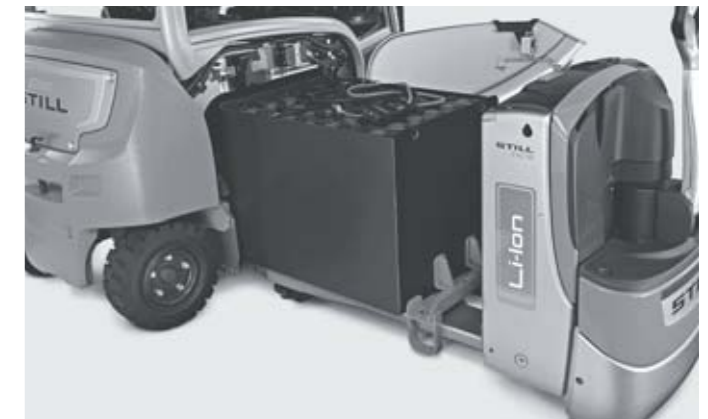
Battery changing with electric pallet truck
