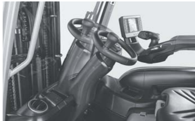
Driver's seat steering column adjustment up/down
