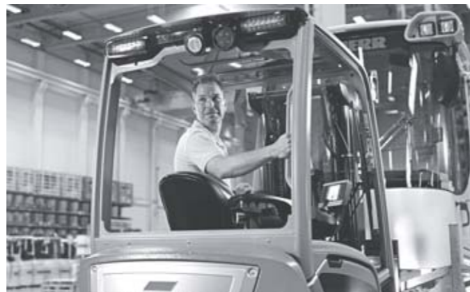
Swivel seat facing to the rear and change of grip on the handle
